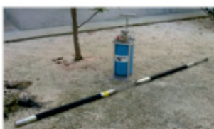
Hydraulic Packer with water pump and fittings
